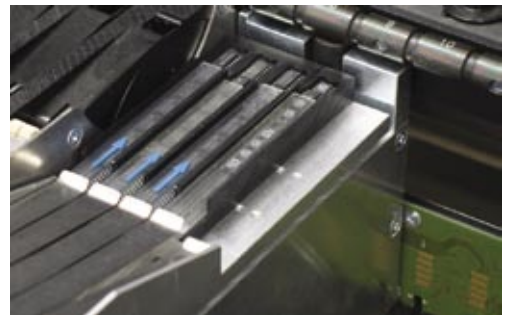
By changing the adapter (black) the stick feeders can quickly be fitted to different component dimensions.
