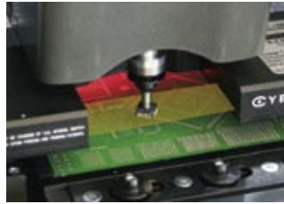
Laser alignment (Cyberoptics) fast and precisely measures all components on their way from feeder to placement location (on the fly).
