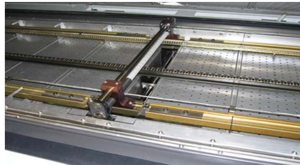
Edge-Hold conveyor and Center board support with center lead-Screw assemblies
